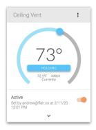
A room tile displays the set point and room temperature for a room. Drag the blue dot to adjust the room's set point. This creates a room "hold". Click the blue "Holding" button to set hold options. The default hold duration is set in Home Settings->System Settings. Toggle the "Active" switch to set the room to Inactive. Flair follows "Away Settings" for inactive rooms. Tap the arrow twiew Puck and Smart Vent status. Tap the 3-dot menu, then select "Stats" to view helpful room statistics.
